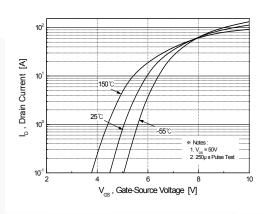
Figure 2. Transfer Characteristics
