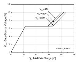
Figure 6. Gate Charge Characteristics
