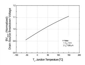
Figure 7. Breakdown Voltage Variation vs. Temperature
