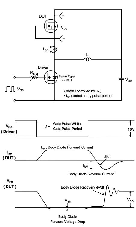
Figure 15. Peak Diode Recovery dv/dt Test Circuit & Waveforms
