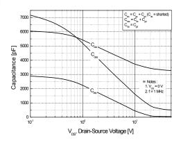
Figure 5. Capacitance Characteristics
