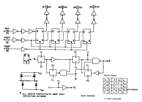
Fig. 1 - Logic diagram (1 register).
