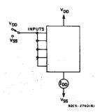
Fig. 10 — Quiescent device current test circuit.
