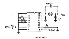
Fig. 9 - Power dissipation test circuit.
