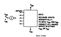
Fig. 12 - Input current test circuit.
