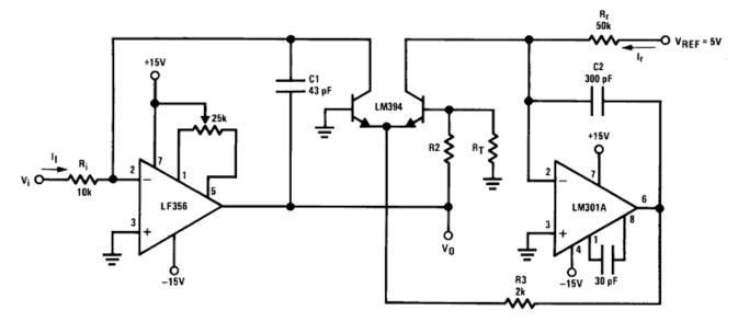
Figure 25. Fast Logarithmic Converter
