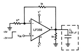
Figure 34. Driving Capacitive Loads
