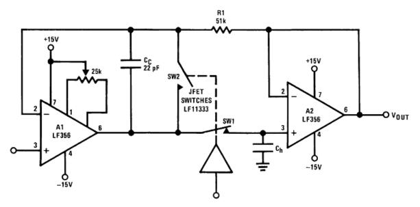
Figure 32. High Accuracy Sample and Hold
