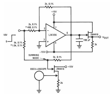
Figure 23. Settling Time Test Circuit
