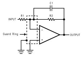
Figure 35. Inverting Amplifier
