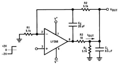
Figure 30. Isolating Large Capacitive Loads
