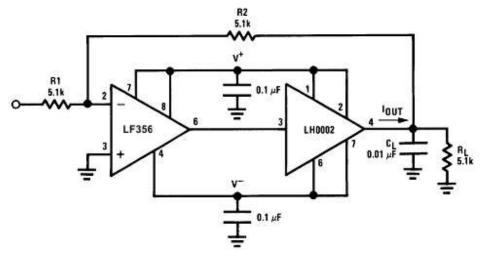
Figure 28. Boosting the LF156 With a Current Amplifier
