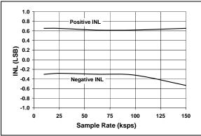
**FIGURE 2-1:** Integral Nonlinearity (INL) vs. Sample Rate.
