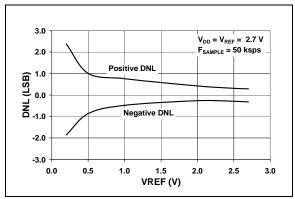
**FIGURE 2-12:** Differential Nonlinearity (DNL) vs.  $V_{REF}(V_{DD} = 2.7V)$ .
