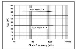
FIGURE 2-35: I<sub>REF</sub> vs. Clock Frequency.
