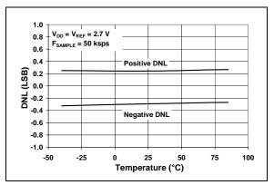
**FIGURE 2-17:** Differential Nonlinearity (DNL) vs. Temperature ( $V_{DD} = 2.7V$ ).
