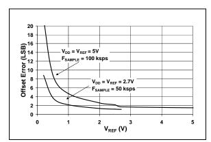
FIGURE 2-18: Offset Error vs. V<sub>REF</sub>
