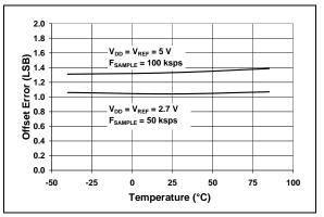
**FIGURE 2-22:** Offset Error vs. Temperature.
