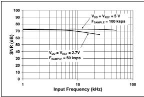
**FIGURE 2-20:** Signal to Noise (SNR) vs. Input Frequency.
