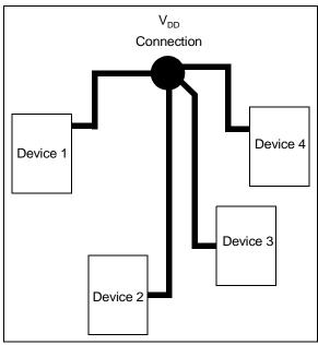
**FIGURE 6-4:**  $V_{DD}$  traces arranged in a 'Star' configuration in order to reduce errors caused by current return paths.
