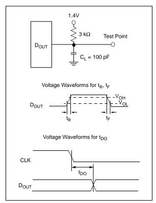
**FIGURE 1-2:** Load Circuit for  $t_R$ ,  $t_F$   $t_{DO}$ .
