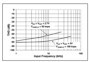
**FIGURE 2-21:** Total Harmonic Distortion (THD) vs. Input Frequency.
