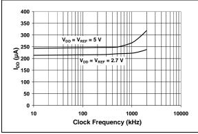
FIGURE 2-32: I<sub>DD</sub> vs. Clock Frequency.
