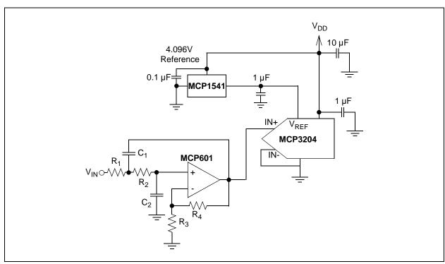
**FIGURE 6-3:** The MCP601 Operational Amplifier is used to implement a second order anti-aliasing filter for the signal being converted by the MCP3204.
