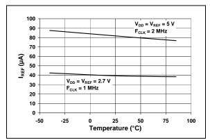
FIGURE 2-36: I<sub>REF</sub> vs. Temperature.
