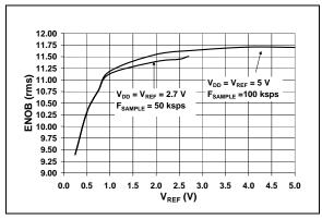
**FIGURE 2-25:** Effective Number of Bits (ENOB) vs.  $V_{REF}$
