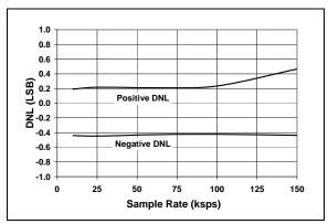
**FIGURE 2-8:** Differential Nonlinearity (DNL) vs. Sample Rate.
