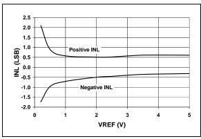
**FIGURE 2-2:** Integral Nonlinearity (INL) vs. V<sub>REF</sub>
