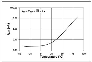
FIGURE 2-38: I<sub>DDS</sub> vs. Temperature.
