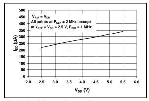
FIGURE 2-31:  $I_{DD}$  vs.  $V_{DD}$ .
