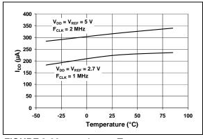
FIGURE 2-33: I<sub>DD</sub> vs. Temperature.
