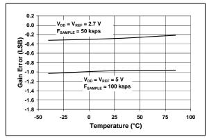
FIGURE 2-19: Gain Error vs. Temperature.
