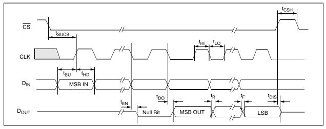
FIGURE 1-1: Serial Interface Timing.
