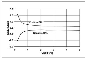
**FIGURE 2-9:** Differential Nonlinearity (DNL) vs. V<sub>REF</sub>
