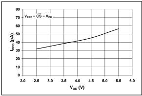
FIGURE 2-37:  $I_{DDS}$  vs.  $V_{DD}$ .
