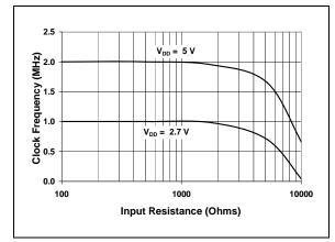
**FIGURE 4-2:** Maximum Clock Frequency vs. Input resistance (R<sub>S</sub>) to maintain less than a 0.1 LSB deviation in INL from nominal conditions.
