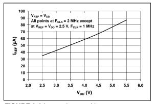
FIGURE 2-34:  $I_{REF}$  vs.  $V_{DD}$ .
