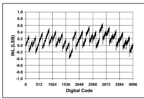
**FIGURE 2-3:** Integral Nonlinearity (INL) vs. Code (Representative Part).
