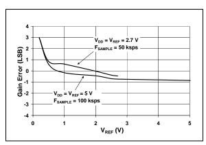
FIGURE 2-15: Gain Error vs. V<sub>RFF</sub>
