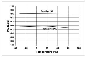
**FIGURE 2-7:** Integral Nonlinearity (INL) vs. Temperature.
