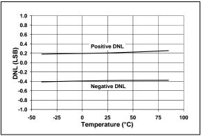
**FIGURE 2-14:** Differential Nonlinearity (DNL) vs. Temperature.
