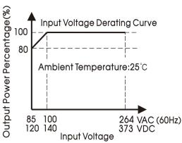
Note: ①With an input voltage between 85-100VAC and a DC input between 120-140VDC the output power must be derated as per the temperature derating
