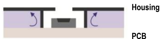
Figure 12. The sensor is isolated from the air inside the housing, which minimizes the impact of the air inside the housing on the sensor.
