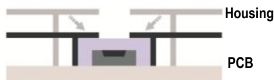
Figure 13. Small measurement dead zone helps the sensor to quickly and comprehensively detect environmental changes.
