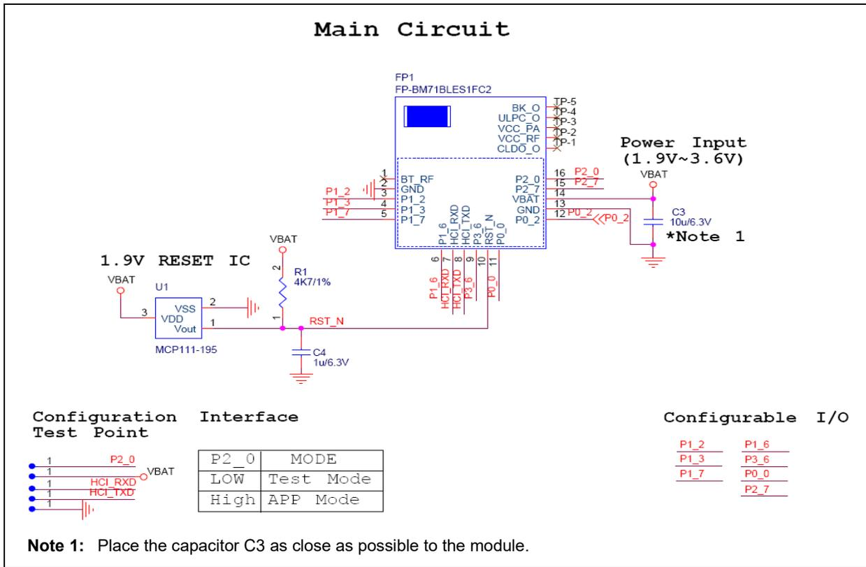
**FIGURE 2-8: BM71BLES1FC2 REFERENCE CIRCUIT - OPTIONAL**
