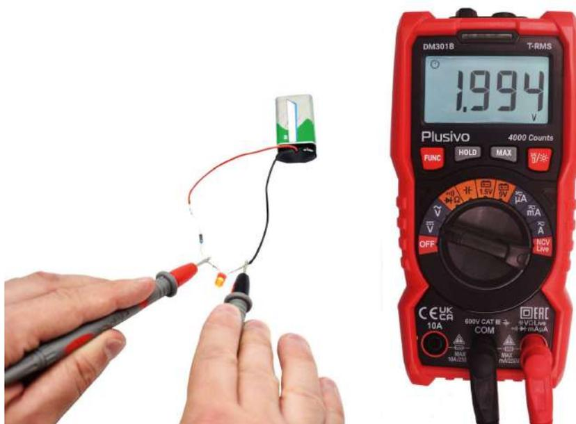
The measured voltage in this figure is 1.994 V DC
