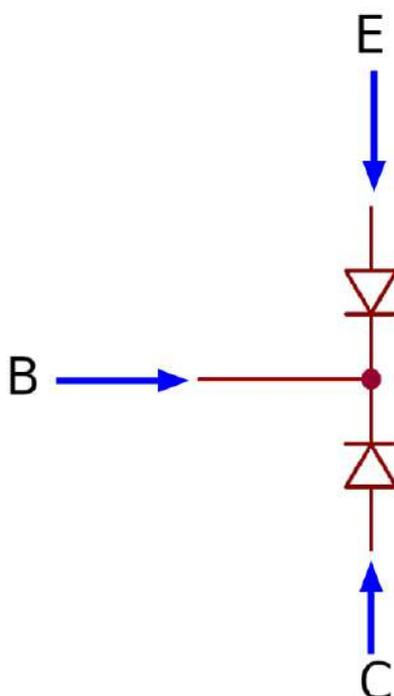
Now, we can test the PNP transistor as 2 diodes. To test the first diode (B - E), we need to connect the black probe to the cathode which is the base of the transistor and connect the red probe to the anode which is the emitter of the transistor.
