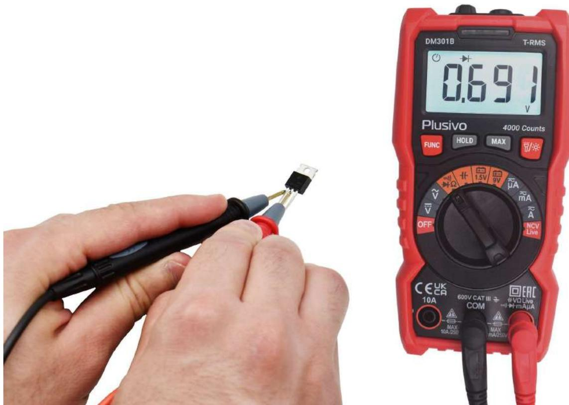
**The measured forward voltage is 0.691 V.**
