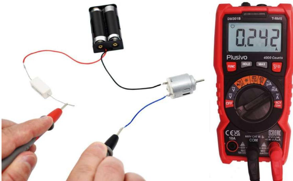
The measured current in this figure is 242 mA.
