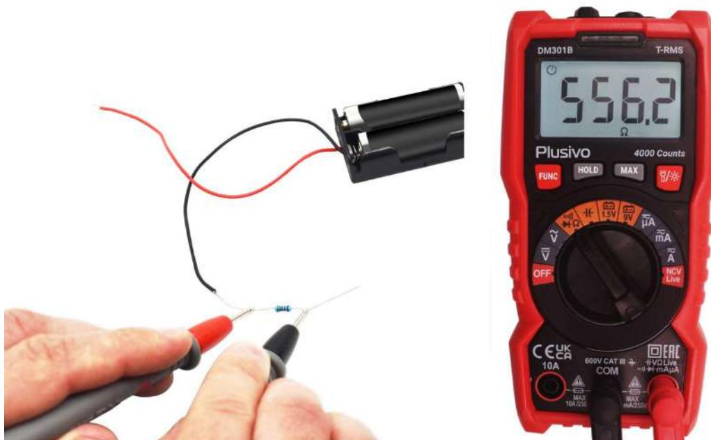
The measured resistance in this figure is **556.2 Ω**.
