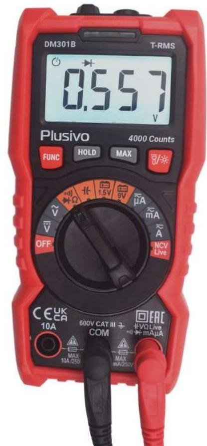
The measured forward voltage in this figure is 0.557 V
