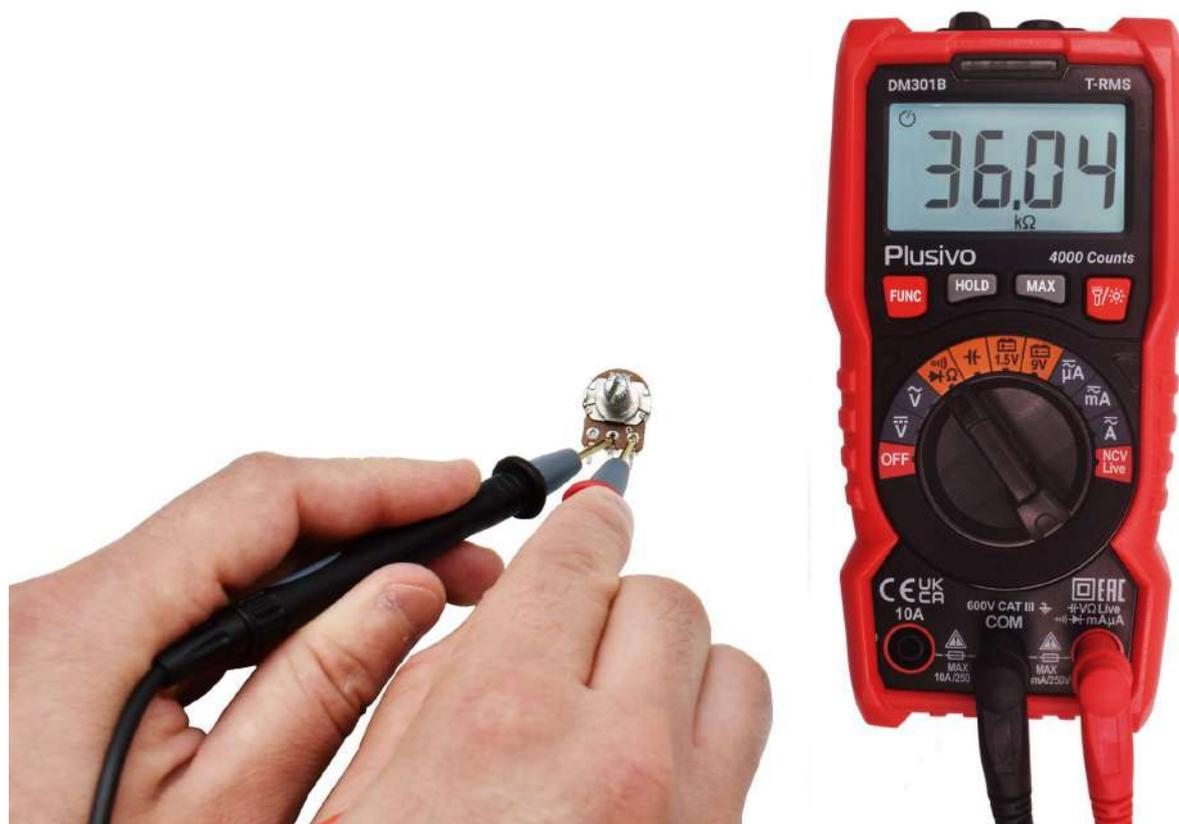
The measured resistance in this figure is 36.04 kΩ.
