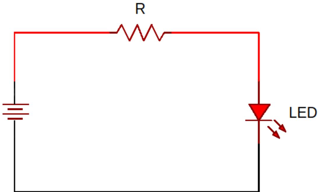
We need to know the voltage around the LED. Usually, a 5 mm LED needs 15 - 30 mA to be in good lighting. After knowing the forward voltage for the LED, it is easy to calculate the resistance.
