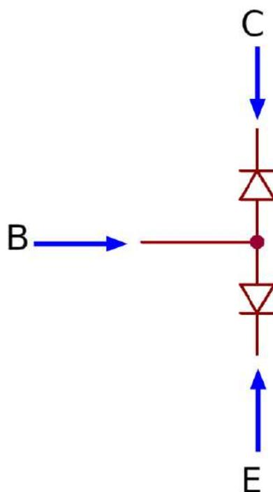
Now, we can test the NPN transistor as 2 diodes. To test the first diode (B - C), we need to connect the red probe to the anode which is the base of the transistor and connect the black probe to the cathode which is the collector of the transistor.
