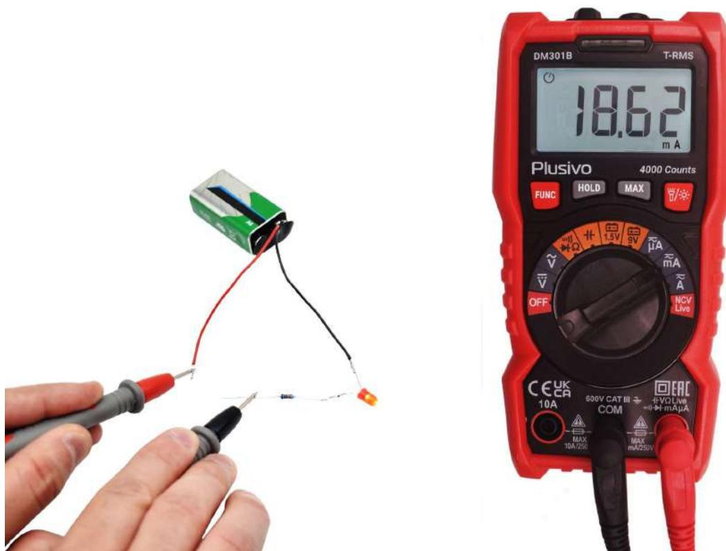
The measured current in this figure is 18.62 mA.
