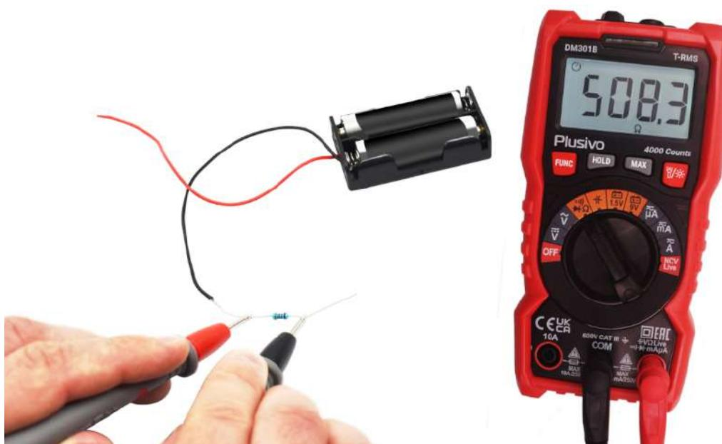
The measured resistance in this figure is 508.3 Ω
