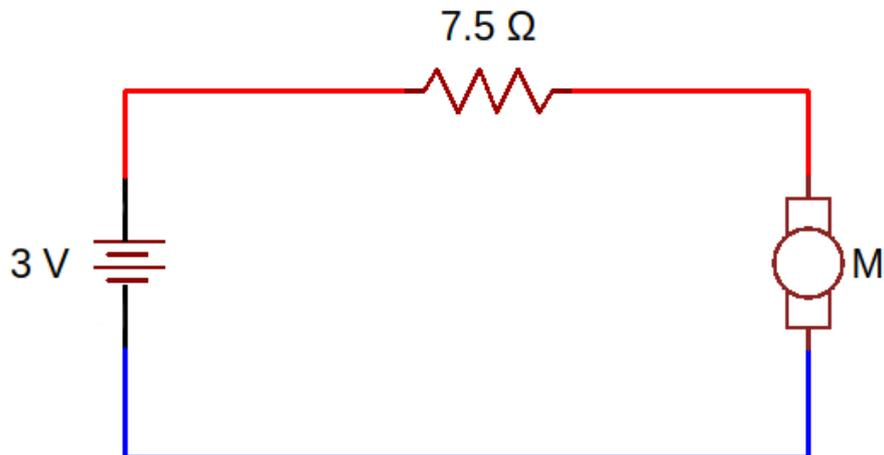
Now, we need to measure the voltage around the  $7.5 \Omega$  shunt resistor using the multimeter.
