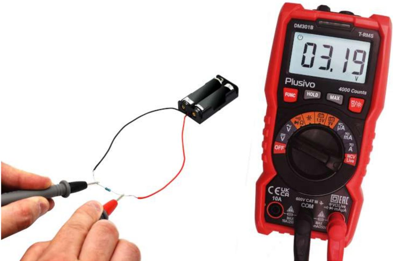
The measured voltage in this figure is 3.19 V DC.
