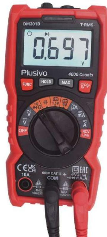
**The measured forward voltage is 0.697 V.**
