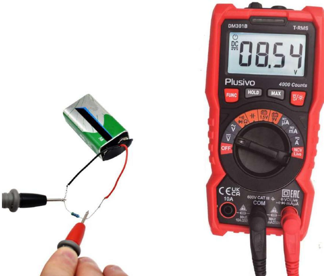
The measured voltage in this figure is 8.54 V DC.
