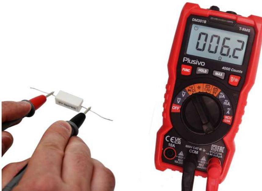
The resistance measured in this figure is 6.2  $\Omega$
