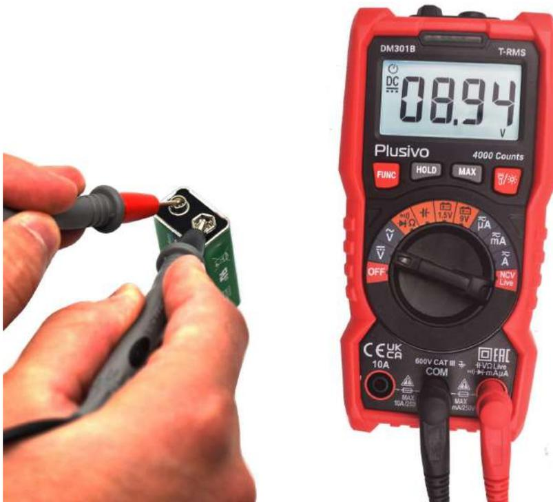
The measured voltage in this figure is 8.94 V DC.
