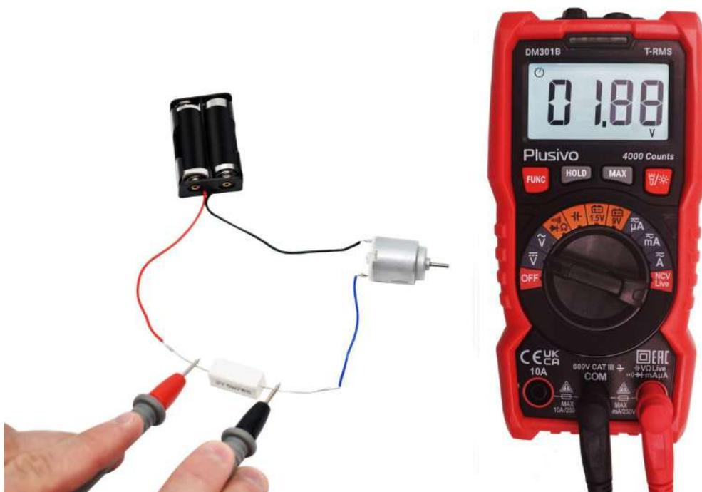
The measured voltage in this figure is 1.88 V DC.
