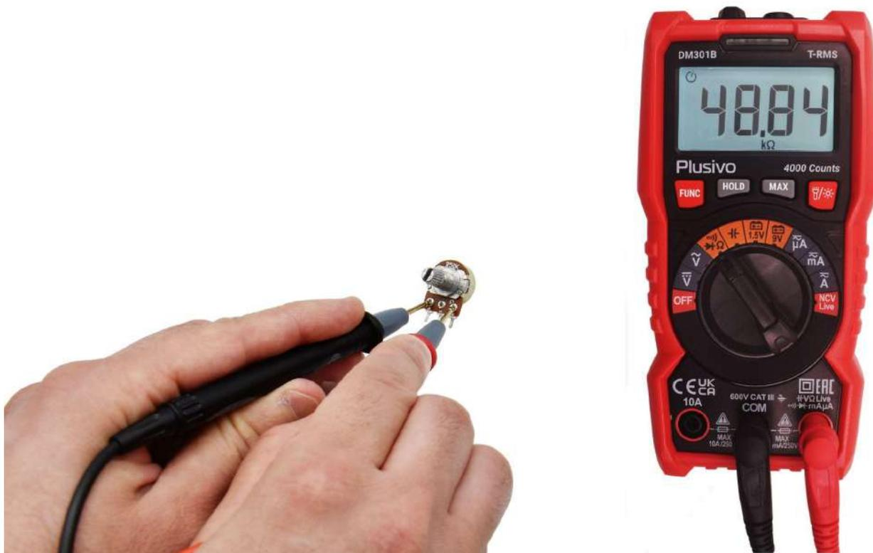
The measured resistance in this figure is 48.84 kΩ.
