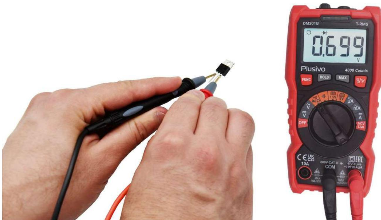
**The measured forward voltage in this figure is 0.672 V.**
