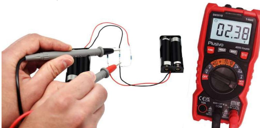
The measured voltage around the 47  $\Omega$  resistor is 0.36 V. Please see the set-up below.
