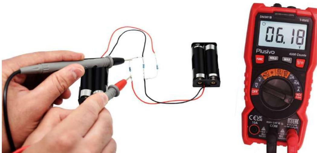
The measured voltage around the 680  $\Omega$  resistor is 2.38 V. Please see the set-up below.
