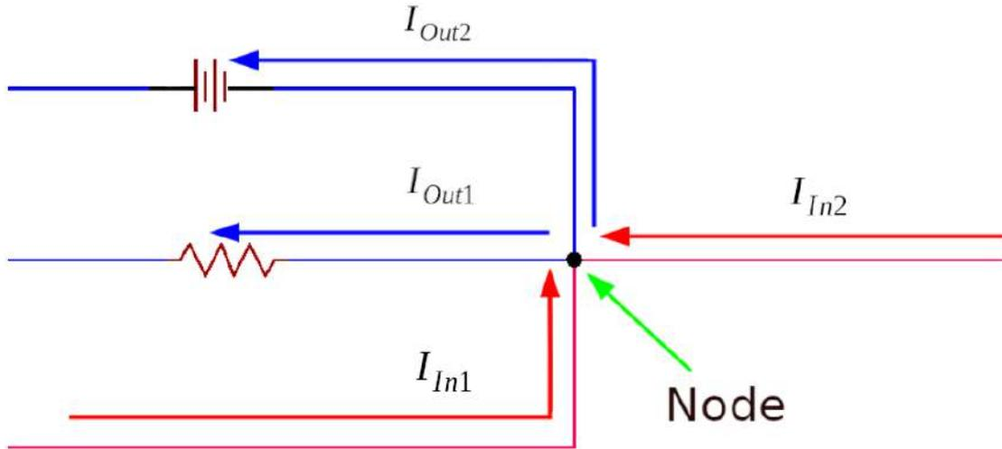
$$I_{In1} + I_{In2} = I_{Out1} + I_{Out2}$$
