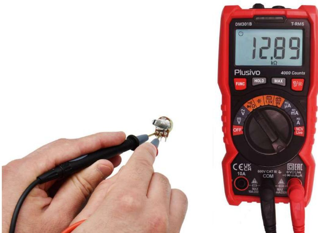
The measured resistance in this figure is 12.89 kΩ.
