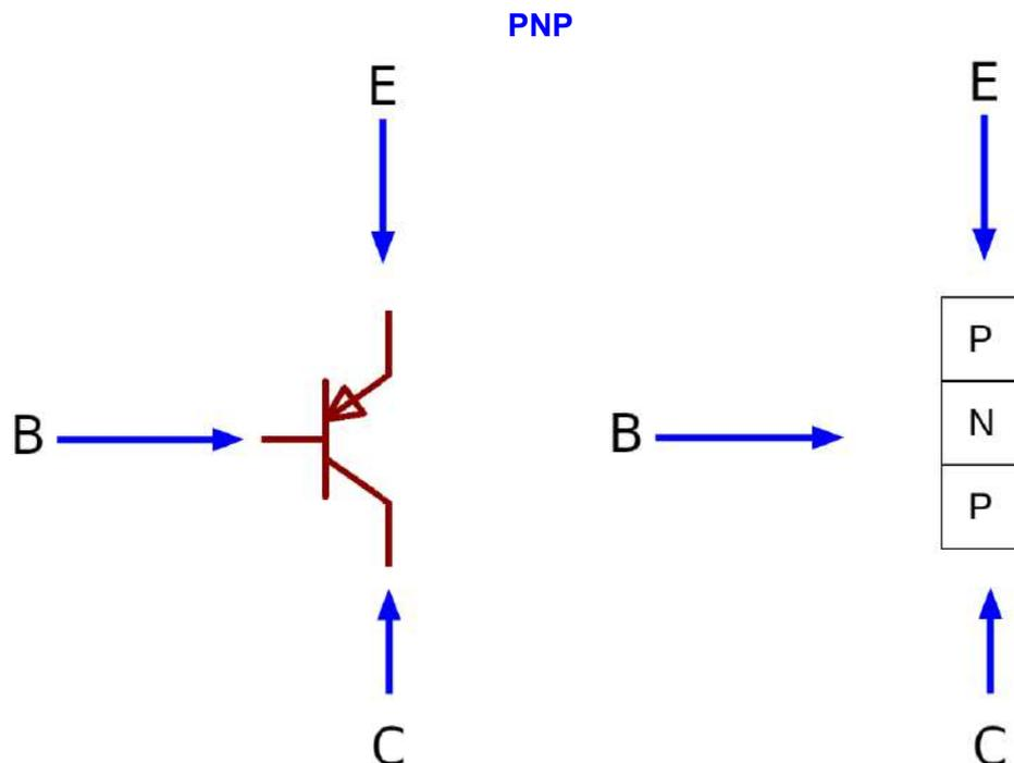
The PNP type consists of two P-Regions separated by N-Region, so we can suppose a diode between B - C and between B - E.
