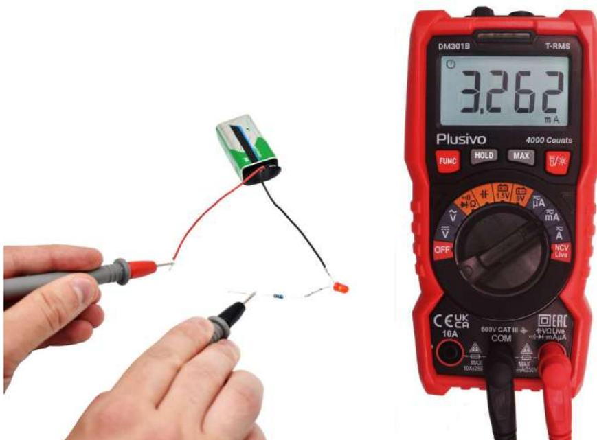
The measured current in this figure is 3.262 mA.
