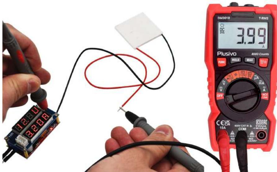
In this set-up, the red probe is inserted in the 10A socket for measuring DC current. The reading is 3.99 A.
