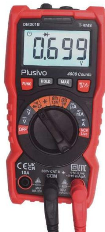
**The measured forward voltage in this figure is 0.699 V.**
