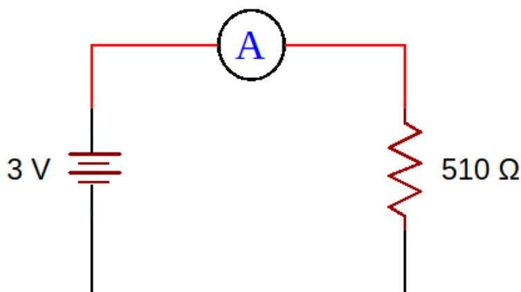
We should read on the screen of the multimeter: **5.88 mA**
