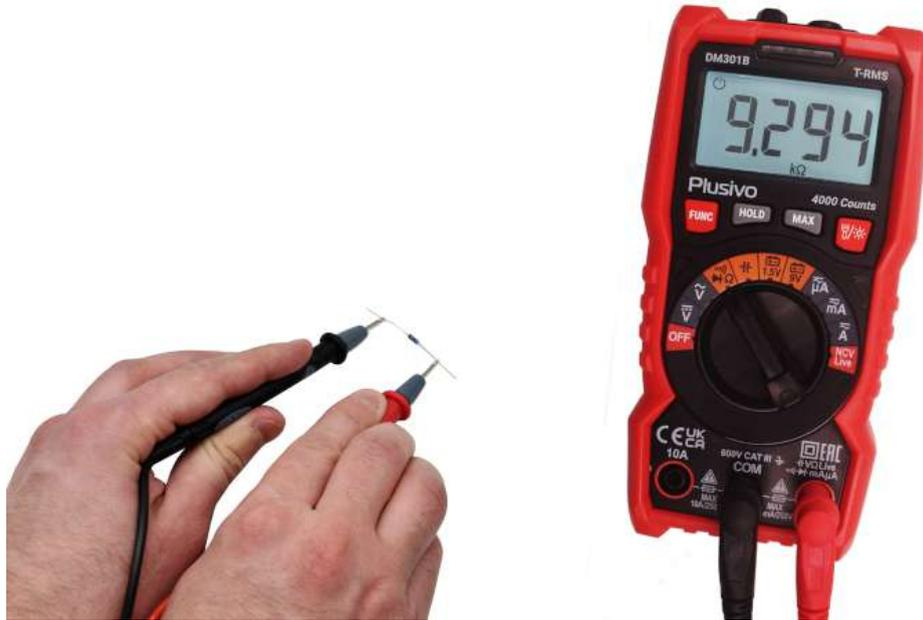
The resistance measured in this figure is 9.294 k $\Omega$
