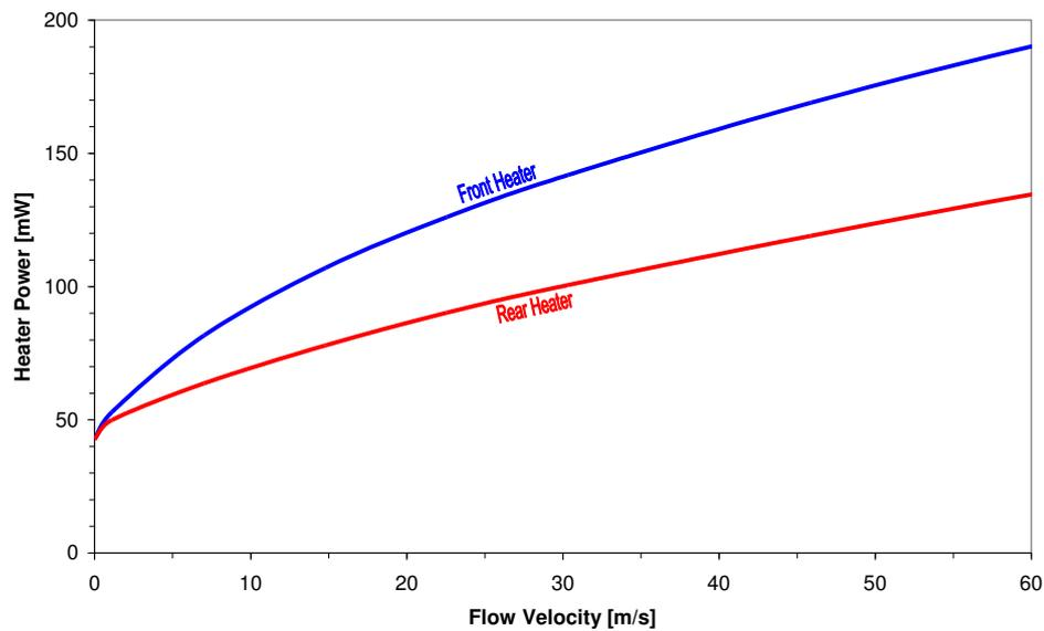
Example of a Power-Flow-Response of the LMM-H03
