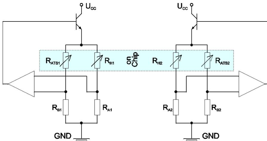
Above is shown an example of a measurement electronics using a Wheatstone-bridge. The resistors R<sub>Ax</sub> and R<sub>Bx</sub> need to be trimmed to operate the heater at a defined over-temperature
