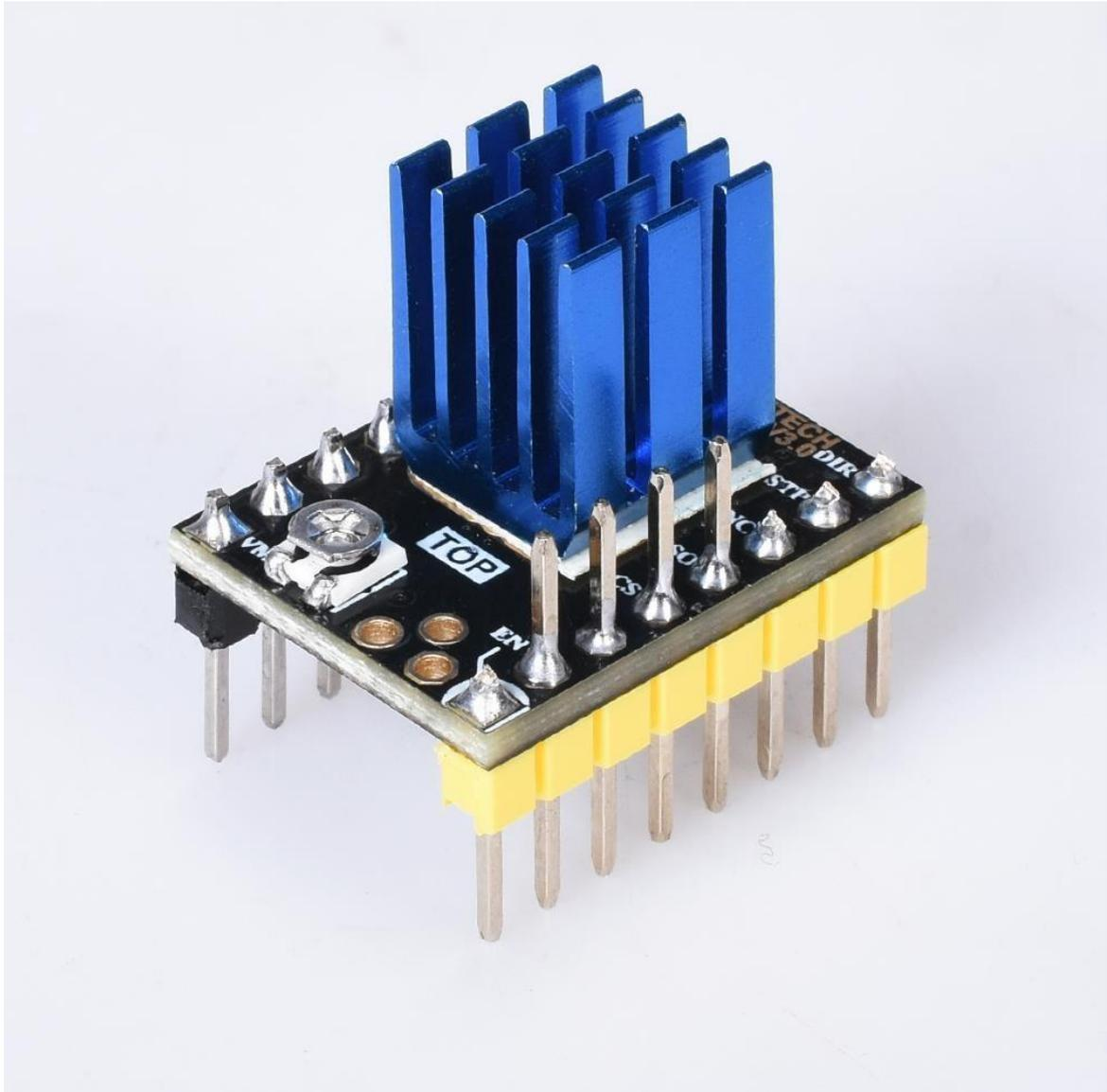
TMC2130 is a high-performance two-phase stepper motor driver chip with a standard SPI interface and a simple step/dir interface. Very low noise, high load driver does not lose step.
