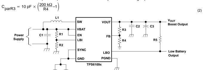
Figure 18. Typical Application Circuit for Adjustable Output Voltage Option
