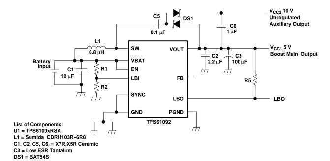
Figure 20. Power Supply Solution With Auxiliary Positive Output Voltage
